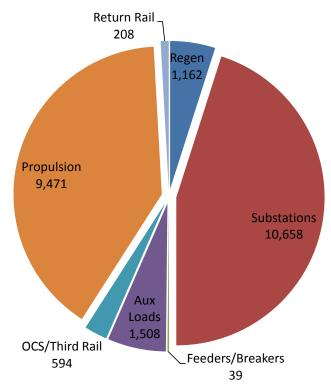
Figure 1: Energy split (in kWh) for a two hour operation scenario on the Gold Line, with actual system settings
