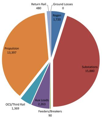
Figure 3: Simulated energy distribution for standard train size (two cars at AW1 and one car at AW0)
