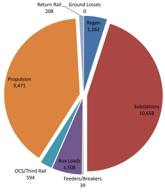
Figure 2: Simulated energy distribution for reduced train size (two cars at AW1)
