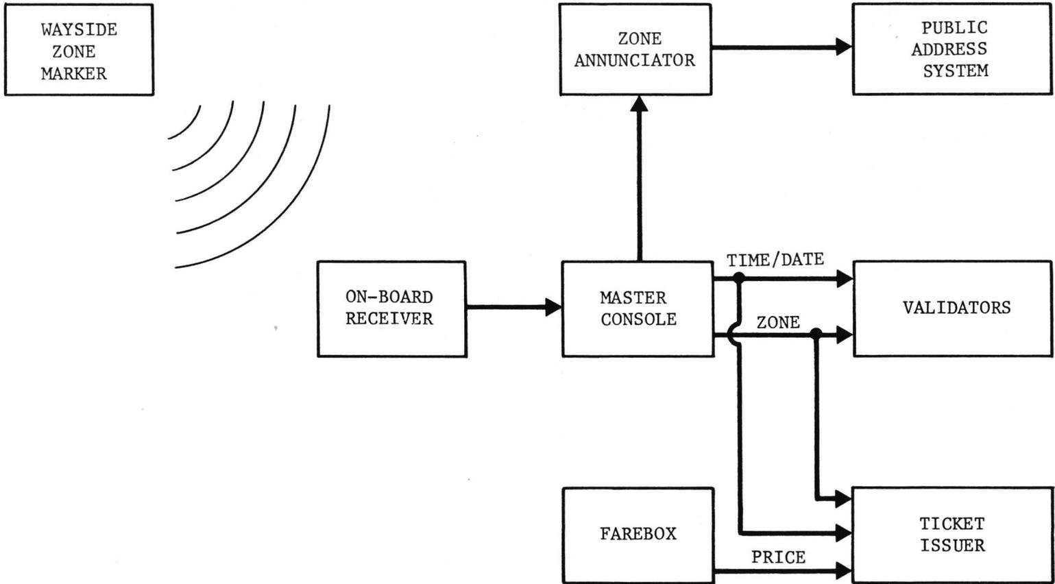
**FIGURE 2. SELF-SERVICE WITH MINIMAL DRIVER INVOLVEMENT**
