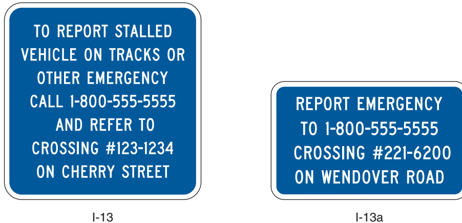
Figure 8B-4. Emergency Notification Signs
