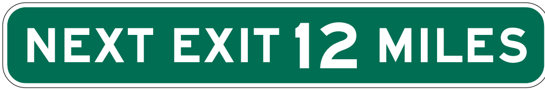
Figure 2E-16. Next Exit Supplemental Advance Guide Signs
