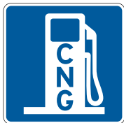
D9-11a Alternative Fuel- Compressed Natural Gas
