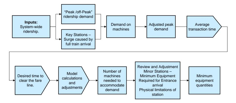
The equipment quantities may be adjusted during the detailed station design process to ensure meeting emergency egress requirements
