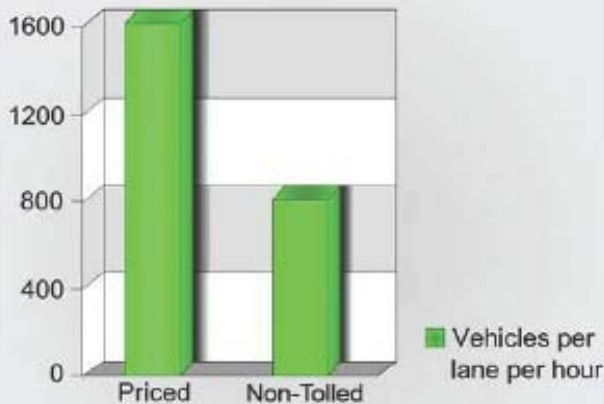
Peak period vehicle throughput during the hour with heaviest traffic, State Route 91 - priced vs. free lanes
