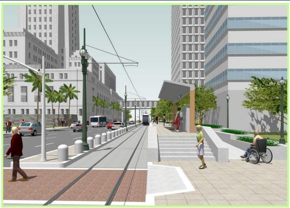
At-grade stations allow pedestrians to move been the sidewalk and the platform quickly without having to navigate stairwells and concourses.
