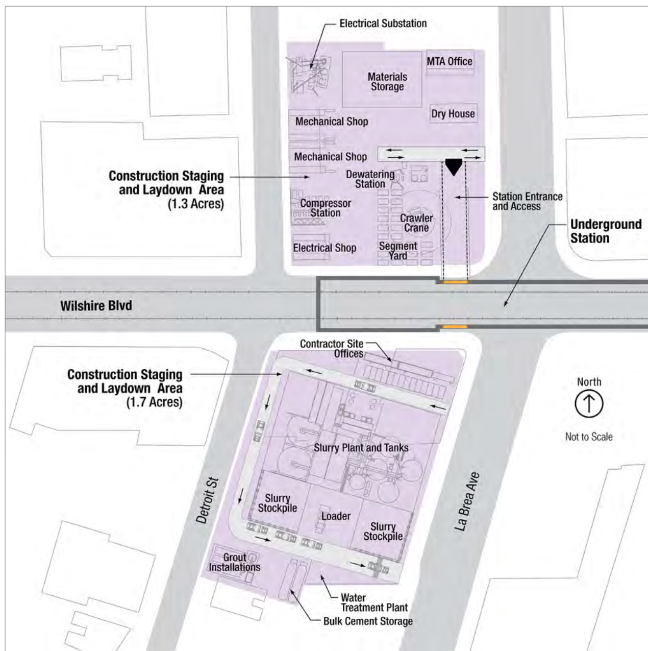
Figure 2-31. Typical Construction Staging and Laydown Site—Wilshire/La Brea
