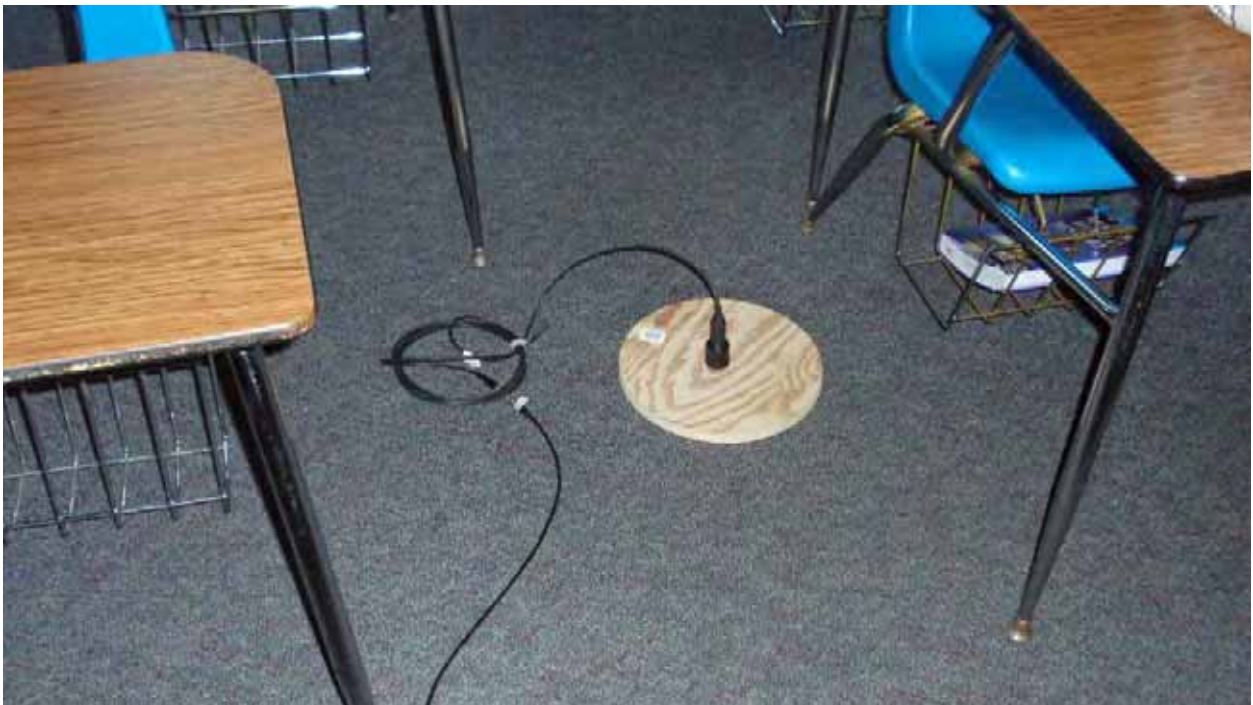
Figure 8-4: Vibration Transducer in Classroom 123
