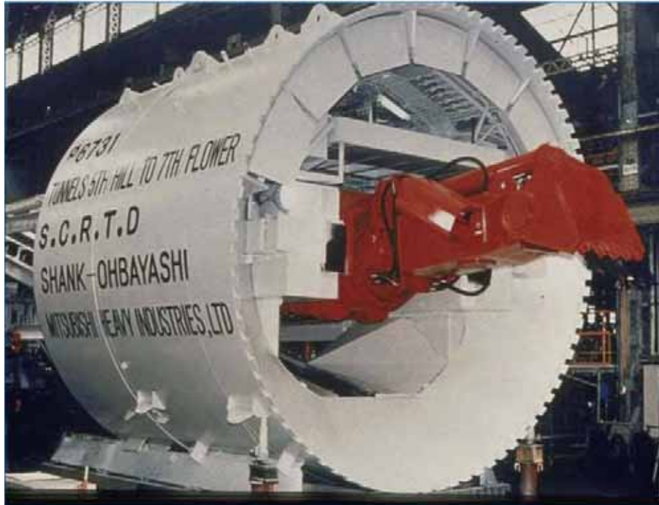
Figure 9-1: Tunnel Shield Used for Metro Segment 1
