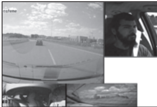
Video data from equipment installed in the vehicles of approximately 3,000 volunteer drivers will be collected over a 2-year period in the SHRP 2 naturalistic driving study.
