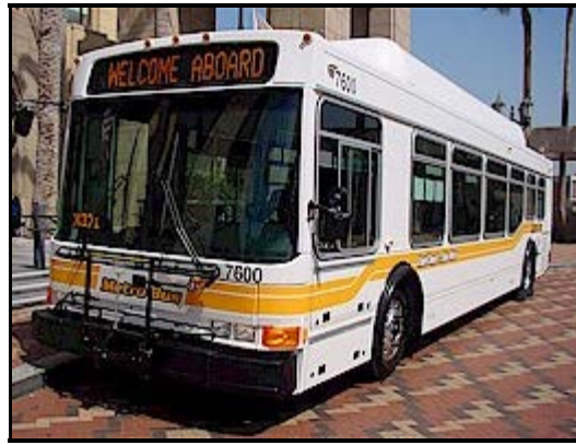
First of a new order of NABI coaches debuts at MTA Sept. 19. Among its innovations: redesigned passenger seats and a CNG fuel tank with 15 percent more capacity.
