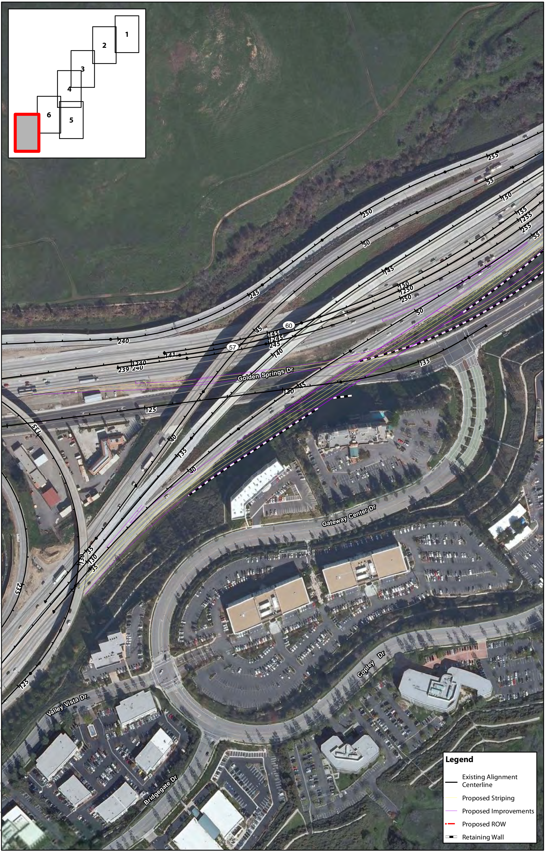
Figure 4-Sheet 7 of 7 Alternative 3, Partial Cloverleaf Interchange Configuration State Route 57/State Route 60 Confluence at Grand Avenue Project
