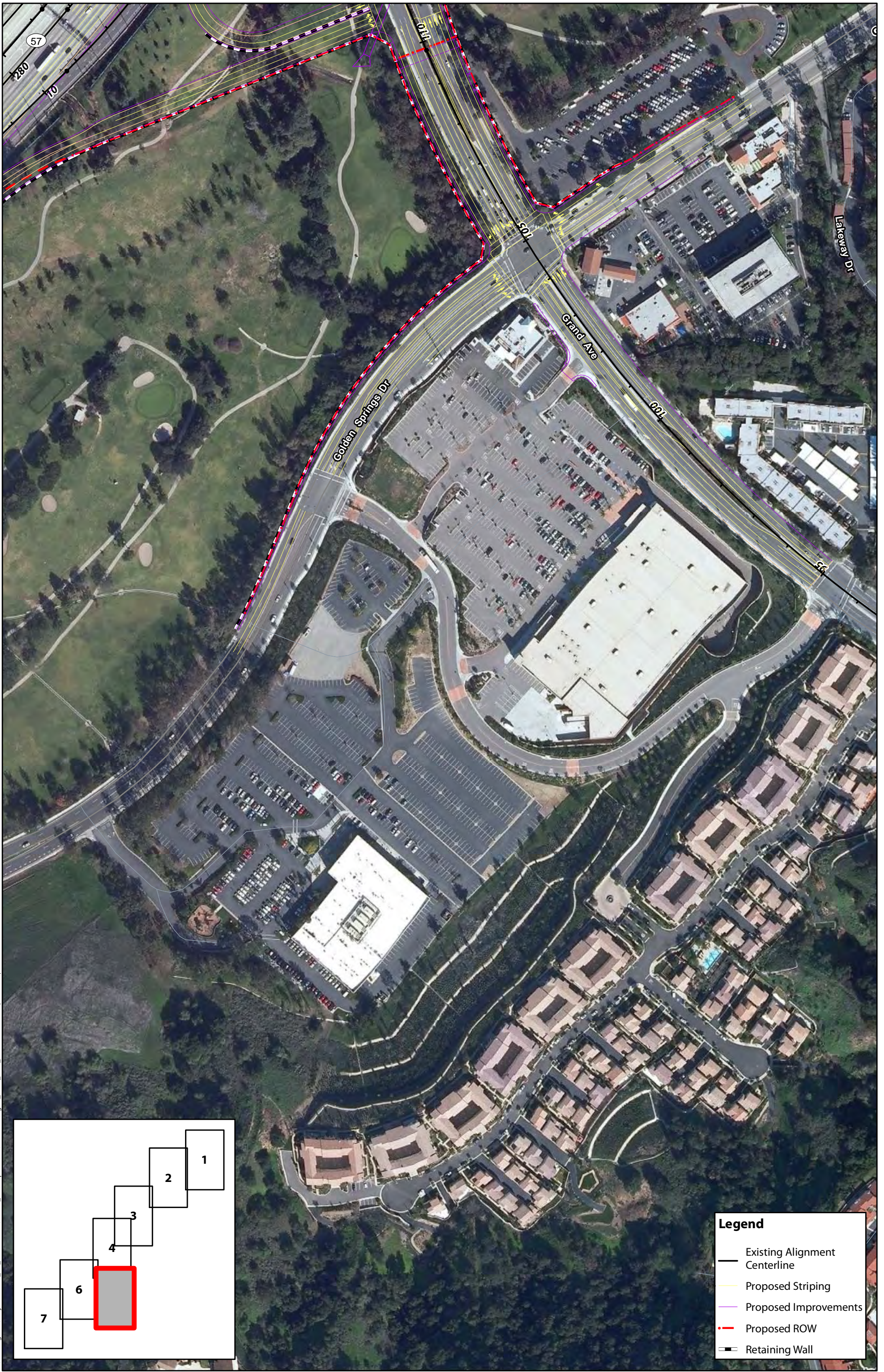
Figure 4-Sheet 5 of 7 Alternative 3, Partial Cloverleaf Interchange Configuration State Route 57/State Route 60 Confluence at Grand Avenue Project
