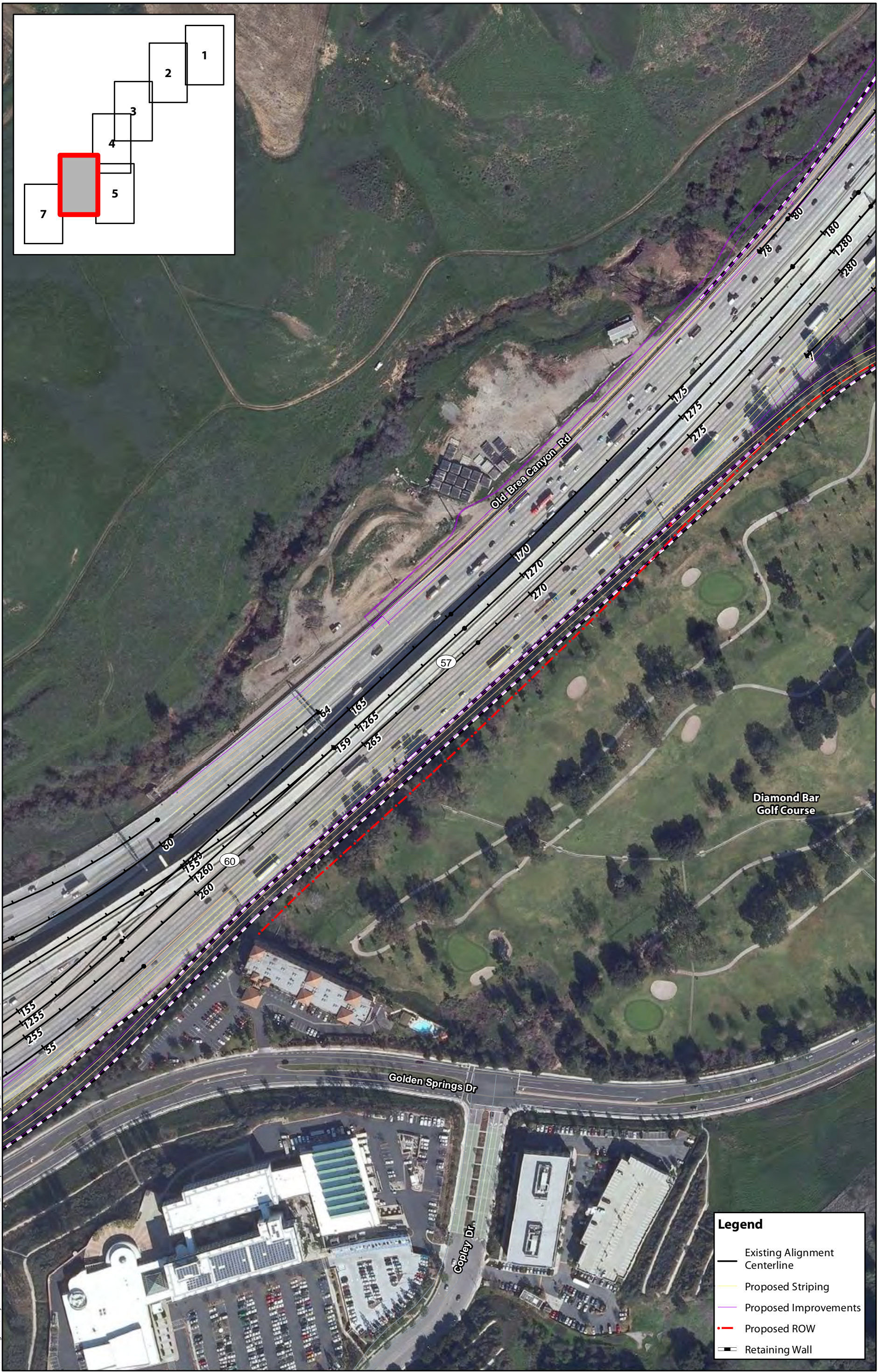
Figure 4-Sheet 6 of 7 Alternative 3, Partial Cloverleaf Interchange Configuration State Route 57/State Route 60 Confluence at Grand Avenue Project
