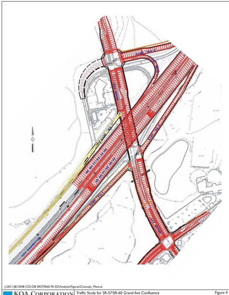
The intersection of Grand Avenue and Golden Springs Drive is reconfigured for double left-turn lanes and a single right-turn lane at all four legs of the intersection (except eastbound, which would retain its current configuration of two right-turn lanes). Grand Avenue in the northbound direction would require median reconstruction and re-striping for 3 through lanes starting approximately 600 feet south of the intersection at Golden Springs Drive.
