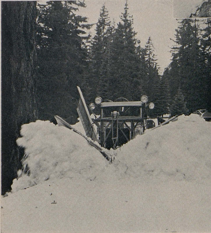
SNOW FIGHTING equipment opening Echo Summit on the Placerville-Lake Tahoe highway. Nos. 1 and 2—Railroad type rotary breaking through a four-foot drift. This machine operates backward into the drifts. No. 3—"V" type push plow bucking a drift. No. 4—View of operating end of the big railroad type rotary doing a little cleaning-up work.
