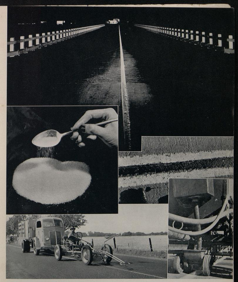
Top photo—Visibility at night of traffic line with beads mixed in lacquer compared with line in foreground painted without them. Left center, beads dropping from spoon are 1/100th of an inch in diameter. Right center—Stripes ragged but bright since 1939. At bottom—striping machine and hopper attachment through which beads are sprayed on the wet paint of stripe
