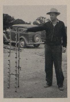
Evans spraybar used ineliminating roadside vegetation alongside State highways
