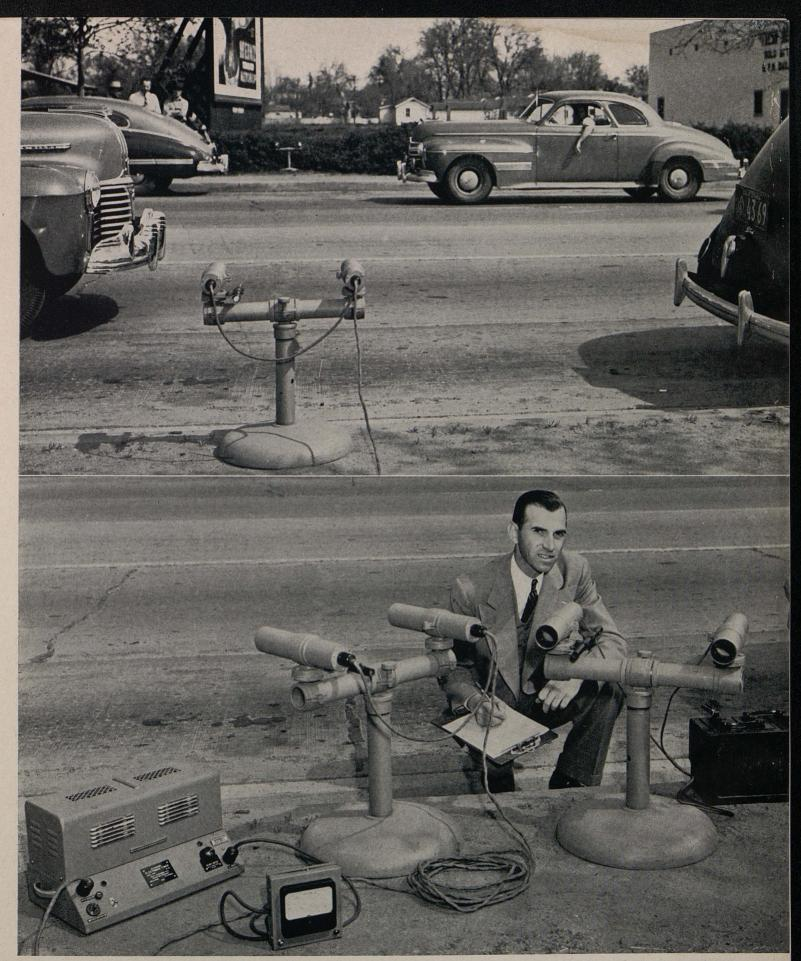
Views of new photo-electric roadside speed timer in action at top. Units of the apparatus are shown below with District Traffic Engineer W. M. Rieth who supervised its development
