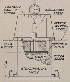
Expansion test for determining swell of bearing value specimens
