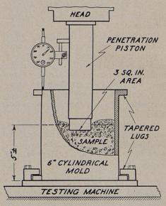
Bearing test equipment for determining resistance of base and subgrade material
