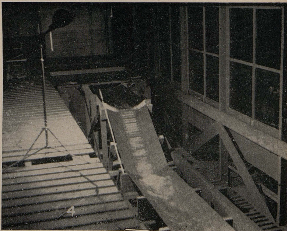
Same dissipating basin dimensions as Fig. 3. Flow is equivalent to 900 c. f. s. in prototype
