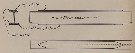
PLATE METHOD OF STRENGTHENING FLOOR BEAMS
