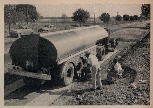
Weighing third axle of type 2s2 gasoline transport combination
