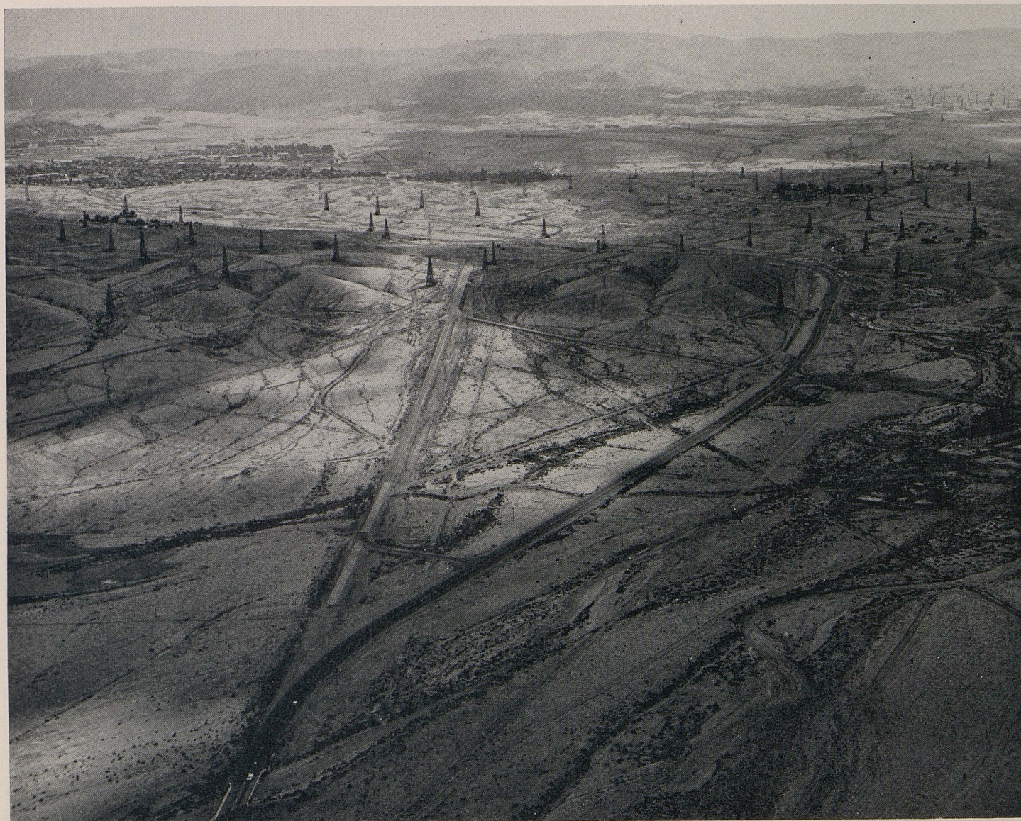
US 399 in Kern County has been relocated around Hill 36. Note the old highway leading directly across the hill (center). Ford City and Taft can be seen in the left background.
