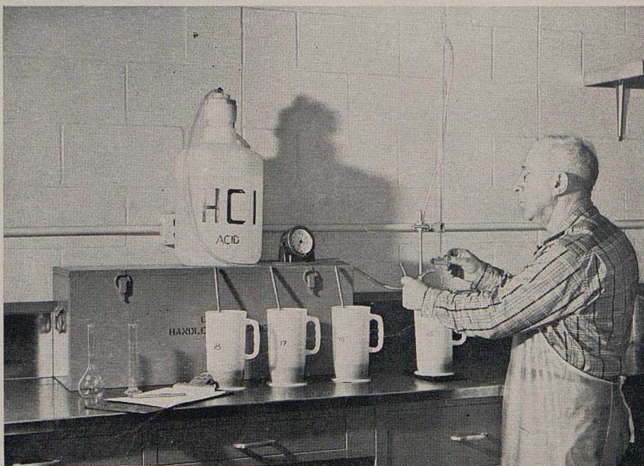
FIGURE 2—Layout for the performance of the constant neutralization procedure is illustrated above.
