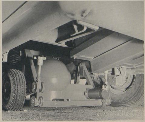
FIGURE 3-The density unit lowered into logging position.
