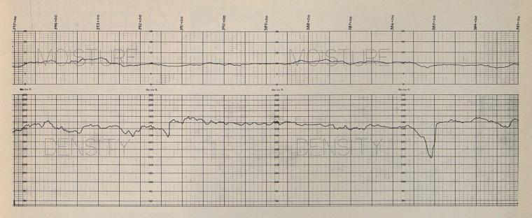
FIGURE 2—Continuous road logger graph of moisture (top) and density (bottom) from Wells Road in Santa Paula.
