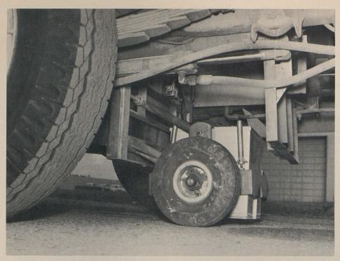
FIGURE 4—The moisture unit lowered into logging position.
