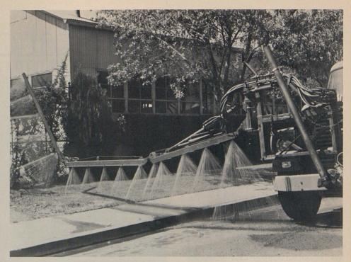
The versatility of the spray proportioner is demonstrated by this positioning of the three eight-foot hinged booms. The irrigation pipe, attached at the center of the truck bumper, is in its travel position.
