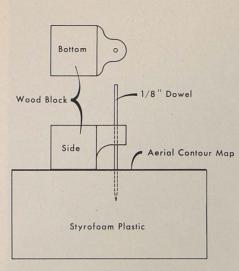
DETAIL OF TOOL USED IN PUNCHING VERTICAL HOLES IN THE STYROFOAM BASE
