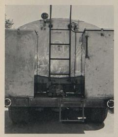
A rear view of the spray proportioner truck shows the two oblong chemical tanks and the oval water tank. The rear steps are retractable.
