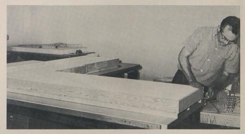
As a base for the models, blocks of styrofoam are combined as desired and framed with wood.
