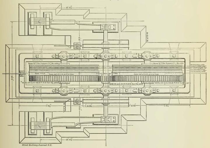
FIG 3.—PLAN OF DRIVING MACHINERY—OTIS ELEVATING RAILWAY.
