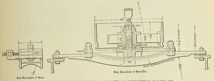
FIG. 6.—CURVE PULLEY AND FRAME—WASHINGTON & GEORGETOWN RAILWAY CO.
