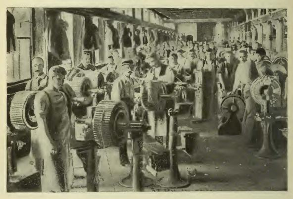
FIG. 8.-WINDING W. P. MOTOR ARMATURES.
