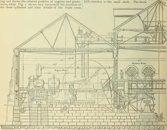
FIG. I .- HALF CROSS SECTION, CENTRAL POWER STATION-WEST END STREET RAILWAY.
