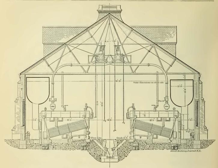
FIG. 7.—CROSS SECTION BOILER ROOM, CENTRAL POWER STATION.
