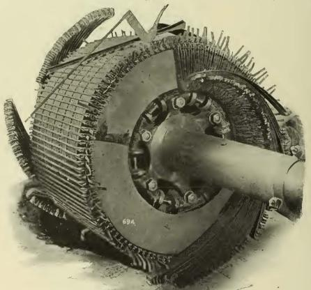
FIG. 2.—METHOD OF WINDING M. P. 500 H. P. GENERATOR ARMATURES (See page 455.)
