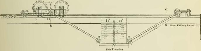
FIG. 10.--UPTON'S TENSION REGULATOR.
