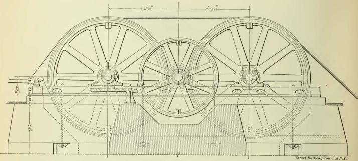
FIG. 2.—SIDE ELEVATION OF DRIVING MACHINERY—OTIS ELEVATING RAILWAY.
