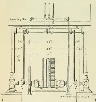
FIG. 1.—END ELEVATION, SHOWING CONTROLLING DEVICES-OTIS ELEVATING RAILWAY.
