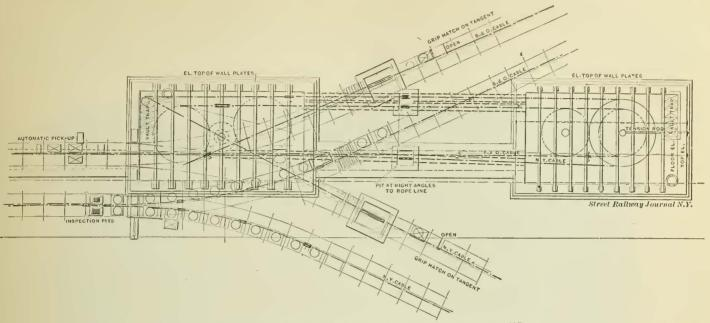
FIG. 4 -AUXILIARY ROPE DRIVE-FOOT OF PENNSYLVANIA AVENUE.
