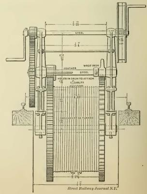
FIG. 9.-TENSION CARRIAGE REEL.
