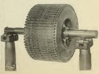
mounted on a gun metal spider similar to that employed in generator construction, and then pressed onto the shaft and secured by a collar nut, when the piece is mounted in a convenient position for filing out the channels, which is done mechanically as shown in Fig. 6.
