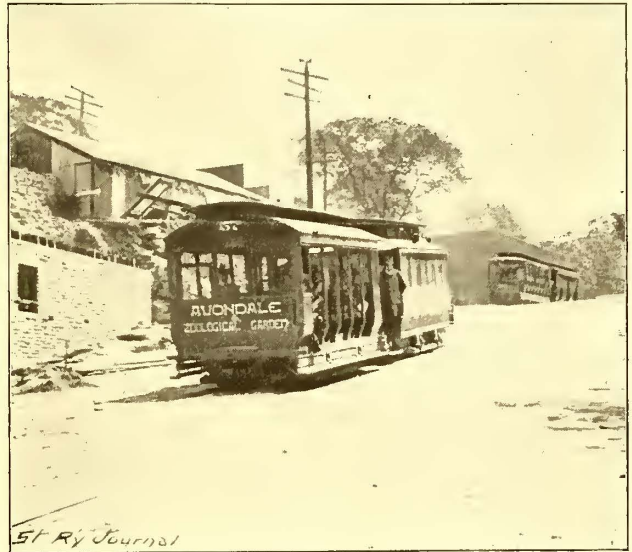
FIG. 13.—COMPOUND CURVE ON 13 PER CENT GRADE—MT. AUBURN CABLE RAILWAY CO., CINCINNATI.
