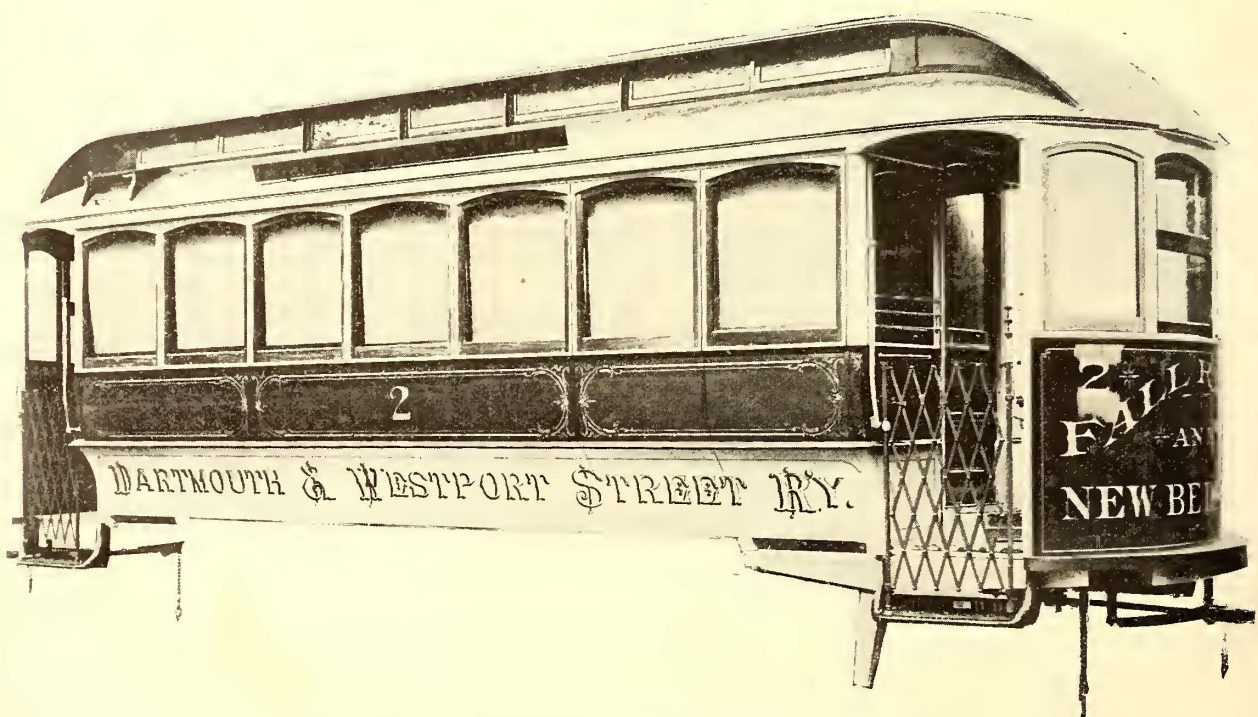
FIG. 2.—CLOSED PASSENGER CAR—DARTMOUTH & WESTPORT STREET RAILWAY.
