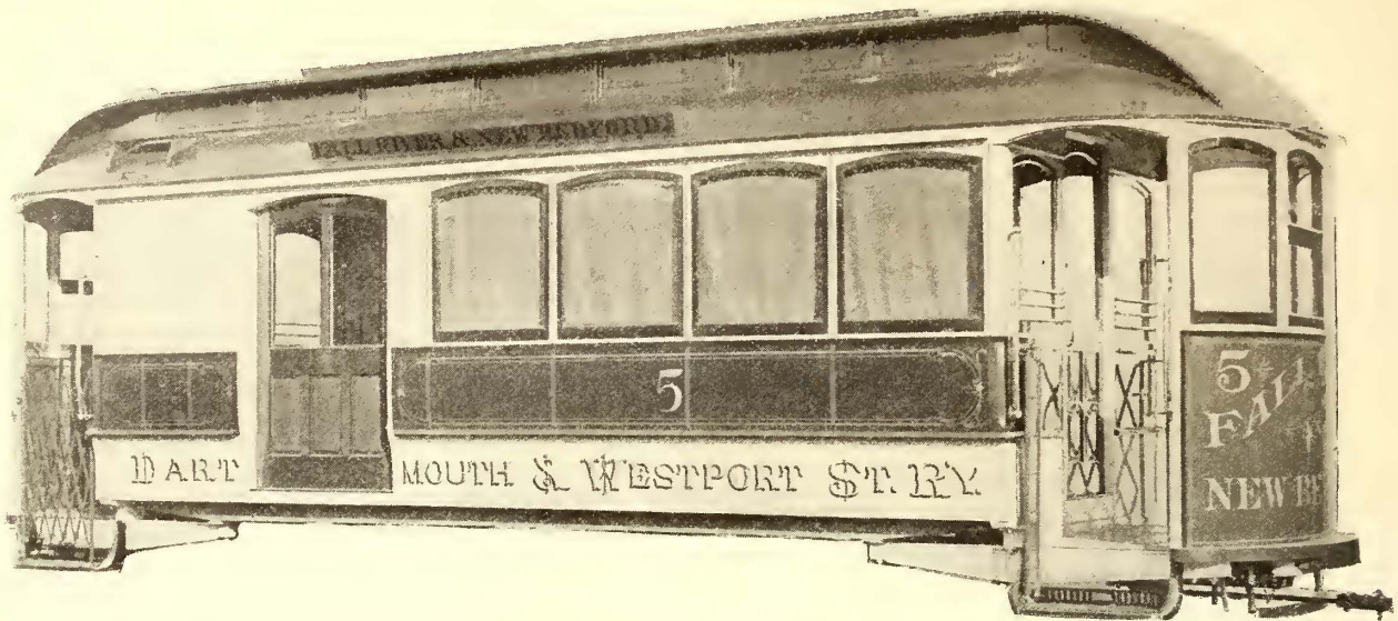
FIG. 1.—COMBINATION BAGGAGE AND PASSENGER CAR—DARTMOUTH & WESTPORT STREET RAILWAY.
