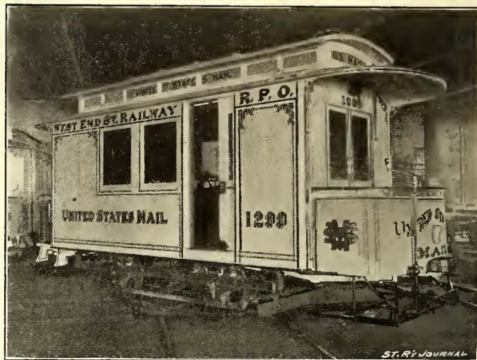
FIG. 3.—NEW MAIL CAR BUILT IN SHOPS OF WEST END STREET RAILWAY.
