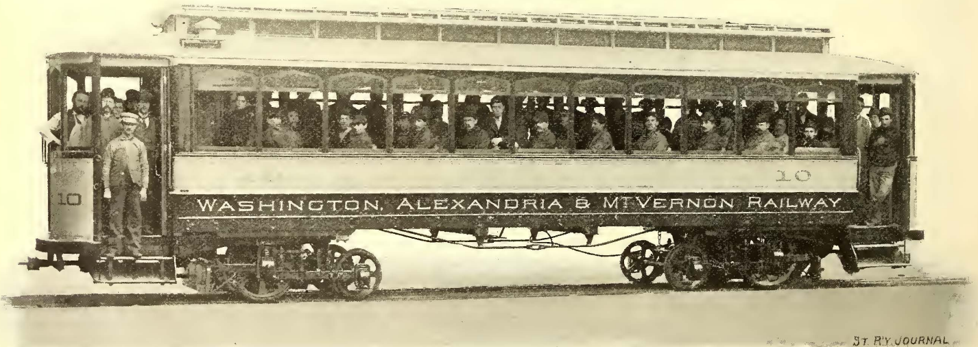
FIG. 4.—DOUBLE TRUCK CAR EQUIPPED WITH AIR BRAKE—WASHINGTON, ALEXANDRIA & MT. VERNON RAILWAY.
