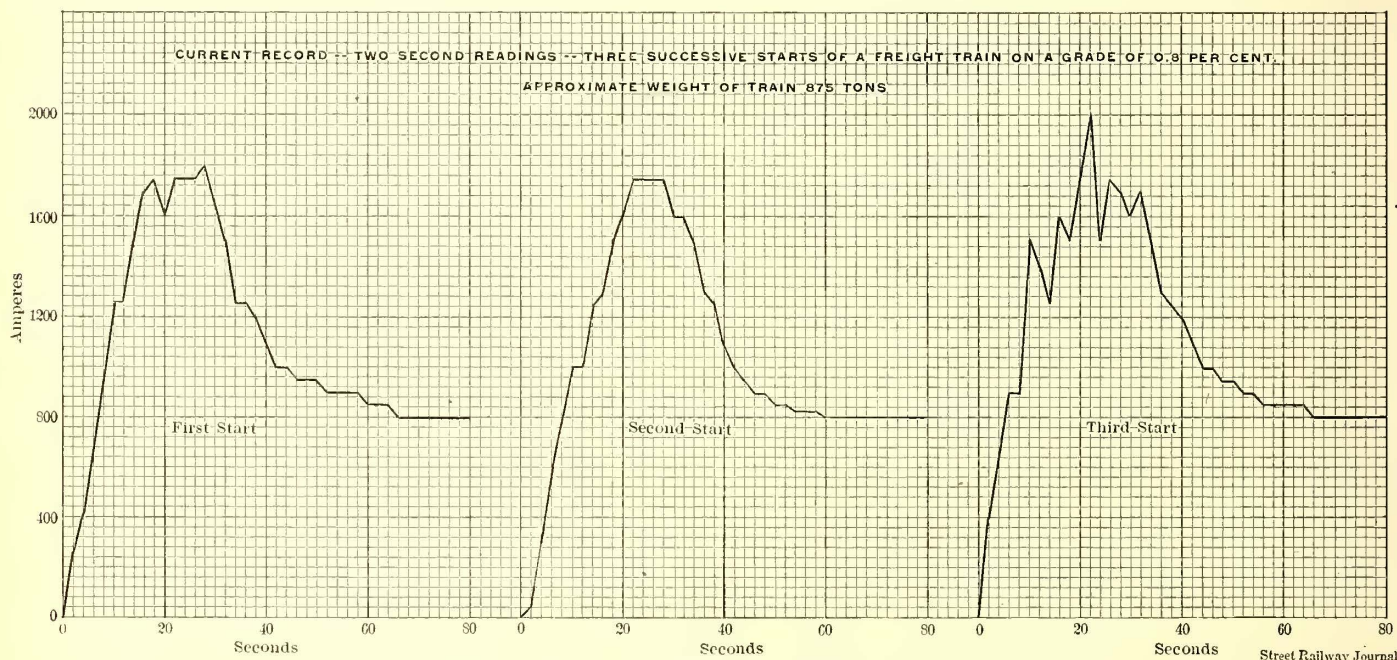
FIG. 2.—CURRENT RECORDS—BALTIMORE & OHIO ELECTRIC LOCOMOTIVE.
