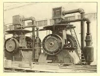
VERTICAL ENGINES WITH COMBINED SEPARATOR AND RECEIVER.
