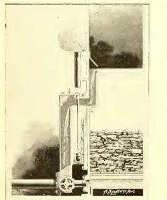
WATER TRAP FOR SEALING OVERFLOW.
