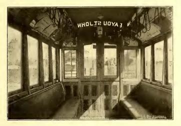
FIG. 8.—INTERIOR OF CAR, SHOWING LIGHTING.
