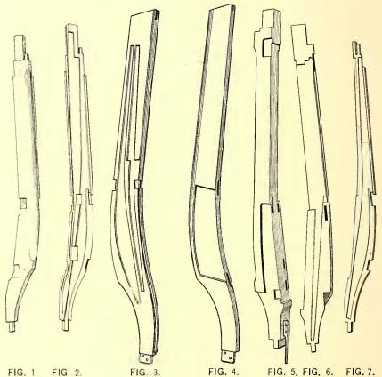
of practice in fastening the plate to the post are shown in Figs. 12 and 7. Fig. 12 has a plain tenon, and is fastened to the plate by the draw pin. This is, perhaps, one of the commonest forms. The Jackson & Sharp Company cm-ploys an entirely different method. It uses what is practically a double tenon (see Figs. 1, 2 and 7), and the plate is not only mortised, but halved upon the post. The double tenon is also used upon the corner post.
