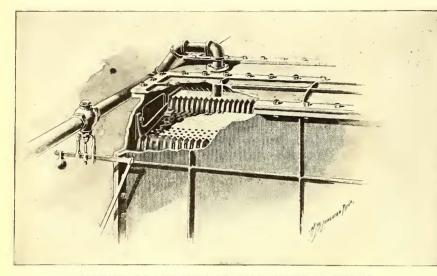
METHOD OF INTRODUCING COLD WATER IN HEATER.
