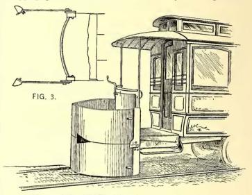
FIG. 2.-CAR FENDER AND PLAN VIEW WHEN OPEN.
