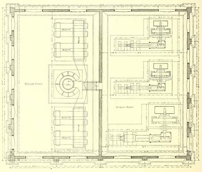
FIG. 10.-PLAN OF STATION AND FOUNDATIONS.
