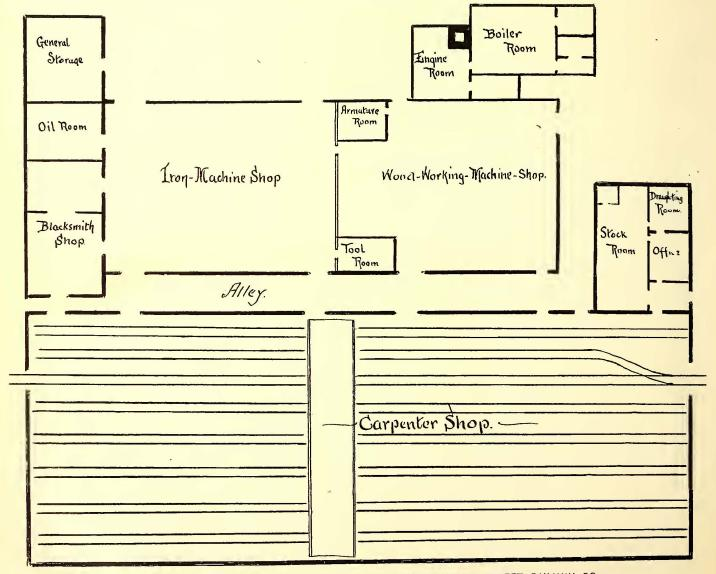
FIG. 1.-DIAGRAMS OF CAR AND REPAIR SHOPS-WEST CHICAGO STREET RAILWAY CO.
