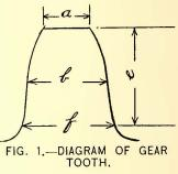
extreme end of one tooth. A few days wear will undoubtedly bring them down to better contact so that an assumption on a worn gear and pinion of one-half the total strain at the end of the tooth would be sufficient.
