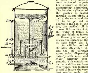
the purifier is heated through steam pipes, 4 and 5, the water and the oil to be purified is poured in the pan at the top, the purified oil is drawn off from faucet 6, the water at faucet I, and the debris at faucet I, 2. Faucet 3 is used only in case the surface of the oil falls below No. 6. As will be noticed the filter illustrated fil-ters the oil through water only, dispensing entirely with waste and other filtering compounds. This constitutes its main difference from
