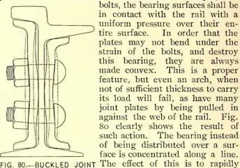
BUCKLED JOINT FIG. 80.-PLATES.
