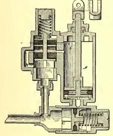
FIG. 3,—SECTION OF AUTOMATIC GOVERNOR FOR COMPRESSOR.
