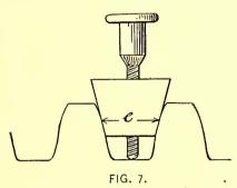
where it comes in contact with the faces of the teeth. Making the angle 14½ degs., brings the point of contact between the wedge and teeth at the pitch line. This gauge also gives a very handy method of determining the amount of wear on a gear in service.
