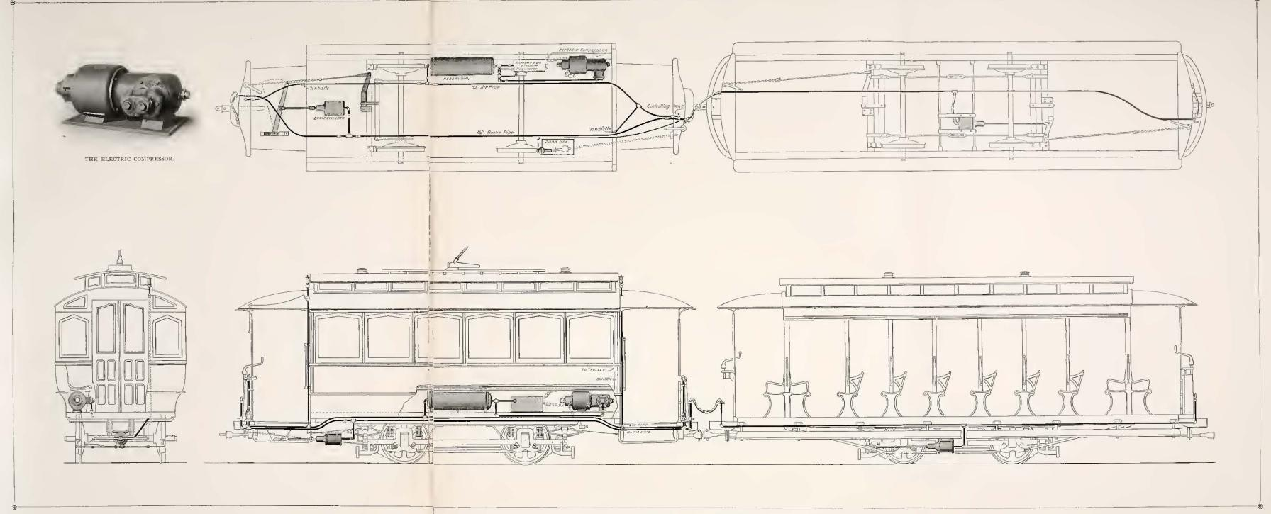
PLAN AND ELEVATION, SHOWING THE AIR BRAKE EQUIPMENT FOR STREET CARS,
