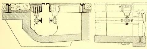
FIG. 5.—CROSS AND LONGITUDINAL SECTION OF CONDUIT AT INSULATOR.
