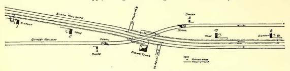
PLAN OF STREET AND STEAM RAILWAY CROSSING PROTECTED BY INTERLOCKING SIGNALS.
