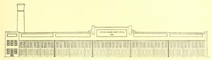
FIG. 9.—FRONT ELEVATION OF CAR HOUSE.
