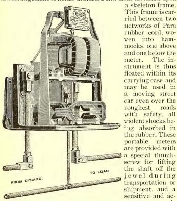
FIG. 3.—WATTMETER WITH CASE REMOVED curate meter is thus insured even
