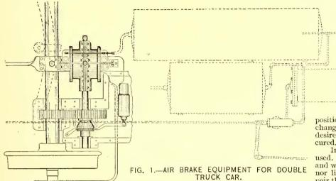
the manner of attaching the compressor to a double truck car, and Fig. 2 that employ-
