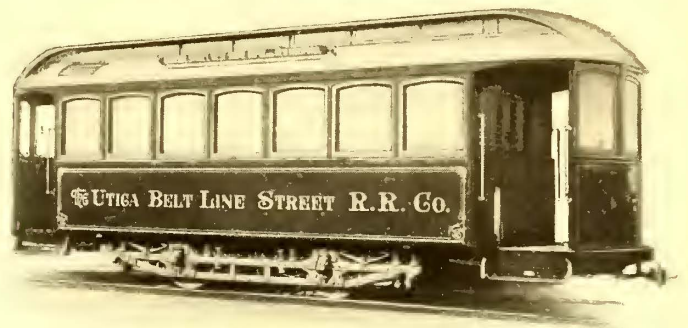
SINGLE TRUCK CENTER AISLE CAR
