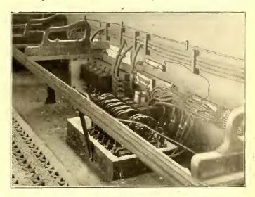
REVERSER AND RELAYS-MULTIPLE UNIT SYSTEM
