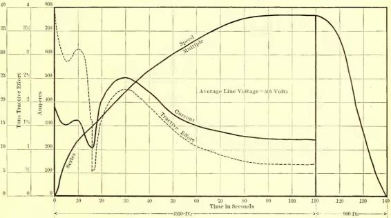
nance accounts FIG. 9-CURVES SHOWING ACCELERATION AND CURRENT CONSUMPTION OF LAKE ST. (CHICAGO) 3 CAR, 58 TON TRAIN-2 150 H. P. MOTORS would therefore be
