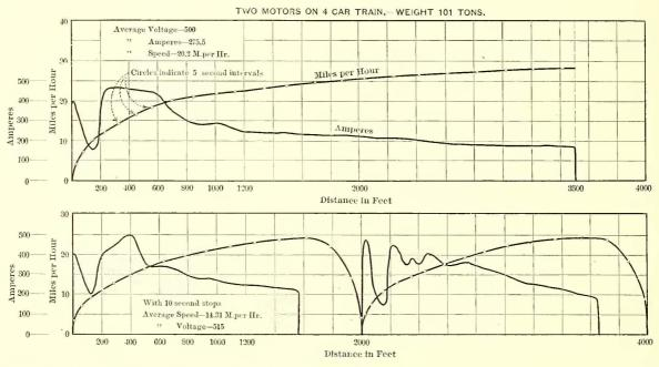
FIG. 7-CURVES SHOWING ACCELERATION AND CURRENT CONSUMPTION OF METROPOLITAN (CHICAGO) TRAIN
