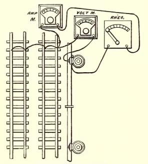
FIG. 4.—DIAGRAM OF CONNECTIONS FOR MEASURING FLOW FROM RAIL TO PIPE
