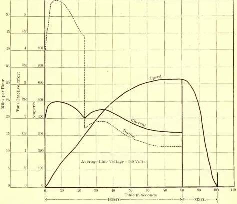
Under the maintenance of equip- FIG. 8-CURVES SHOWING ACCELERATION AND CURRENT CONSUMPTION OF LAKE ST. (CHICAGO) 5 CAR, 90 TON TRAIN-2 150 H. P. MOTORS
