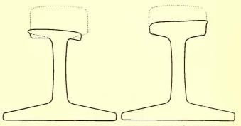
FIG. 2.-RAILS ON CURVE AFTER ONE YEAR'S SERVICE
