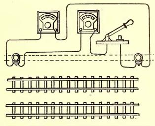
FIG. 3.—DIAGRAM OF CONNECTIONS FOR MEASURING FLOW IN PIPES
