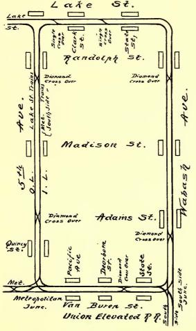
FIG. I-TRACK PLAN OF THE LOOP
