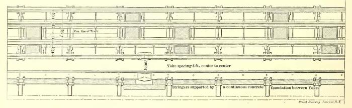
FIG. 4.-PLAN AND SIDE ELEVATION OF NEW CONSTRUCTION
