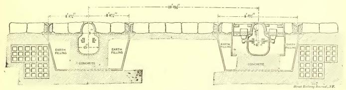
FIG. 6.-SECTION THROUGH ROADBED ON THIRD AVENUE
