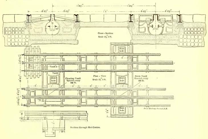
FIG. 1.-PLAN AND SECTIONS OF STANDARD NEW CONSTRUCTION, THIRD AVENUE RAILWAY
