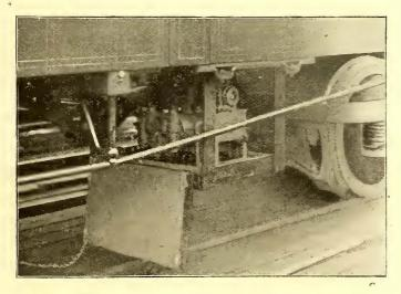
ELECTRIC MOTOR AIR COMPRESSOR
