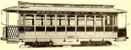
FIG. 2.-CONVERTIBLE CAR USED CLOSED
