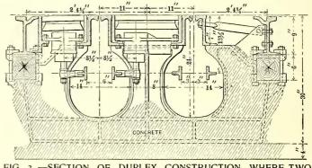
FIG. 3. —SECTION OF DUPLEX CONSTRUCTION WHERE TWO COMPANIES OPERATE OVER SAME TRACK
