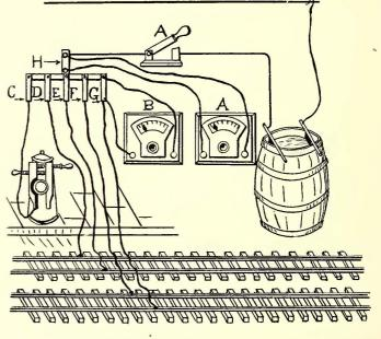
FIG. 5.—DIAGRAM OF CONNECTIONS FOR MEASURING RELATIVE VALUE OF RETURNS
