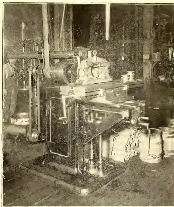
FIG. 1—TOOL FOR CUTTING GROOVES IN TROLLEY WHEELS
