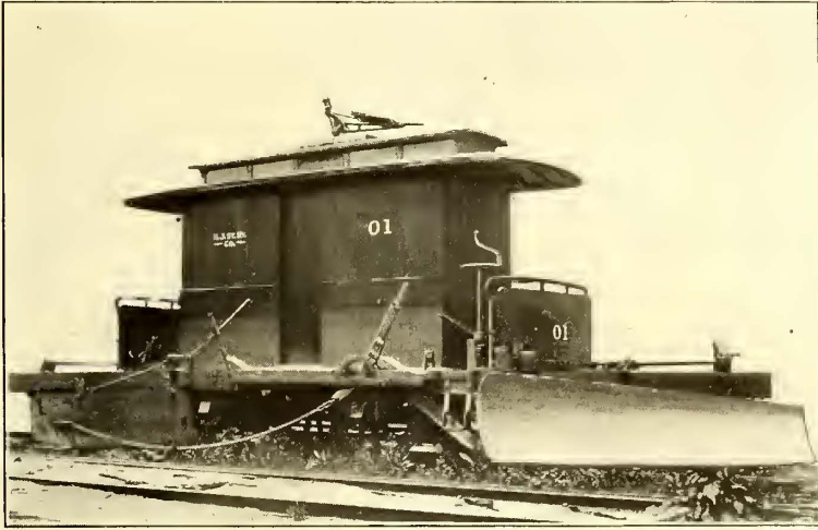
FIGS. 7 AND 8.—SNOW PLOW, NORTH JERSEY STREET RAILWAY CO.
