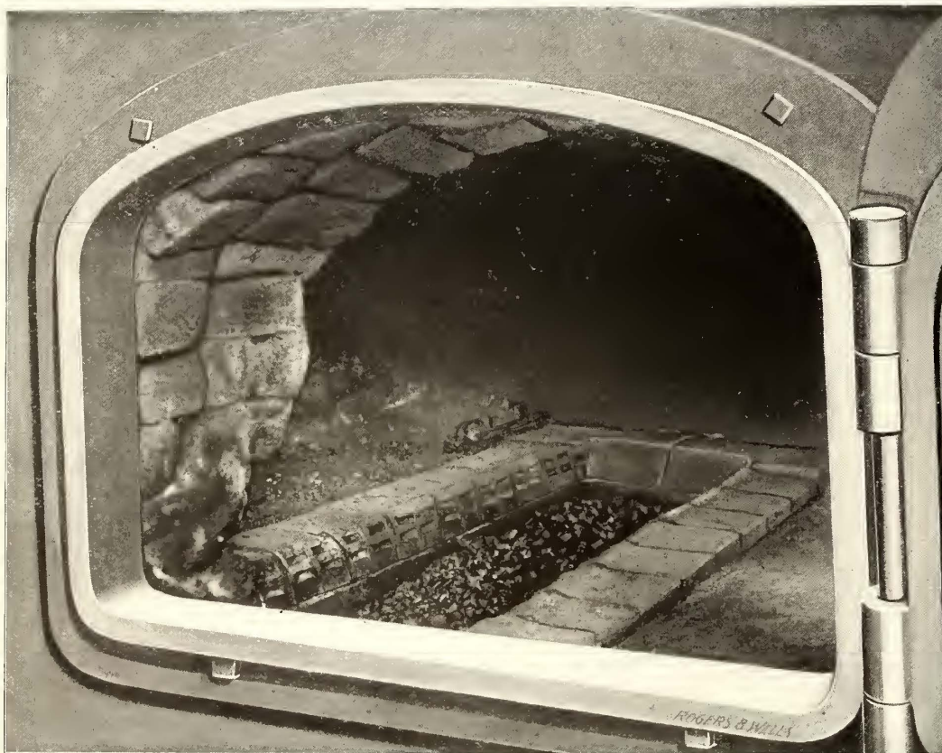
FURNACE AFTER ELEVEN MONTHS' SERVICE
