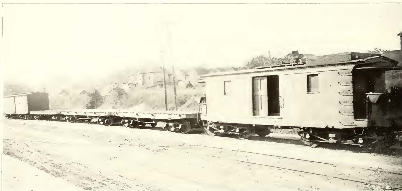
ELECTRIC LOCOMOTIVE ON THE INDEPENDENCE LINE, DRAWING A TRAIN OF FREIGHT CARS
