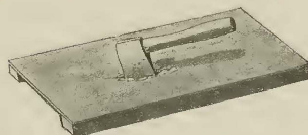
FIG. 615. EFFECT OF INJURY TO PANEL WHEN BACKED WITH "SCRIMS" AND WHEN NOT SO BACKED
