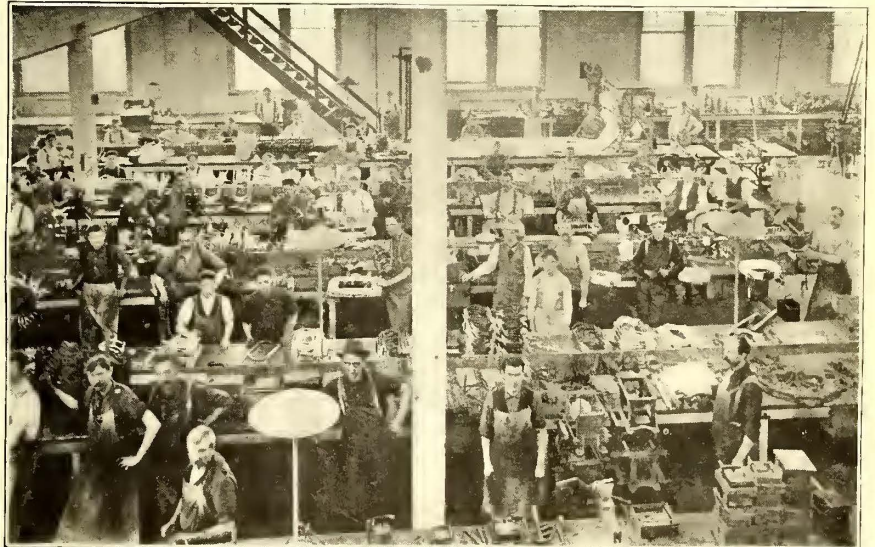
WINDING AND TESTING ARMATURE COILS
