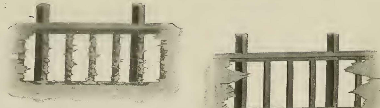
FIG. 618. EFFECT OF GLUE AND LACK OF SAME ON SIDE PANELS WHEN REMOVED
