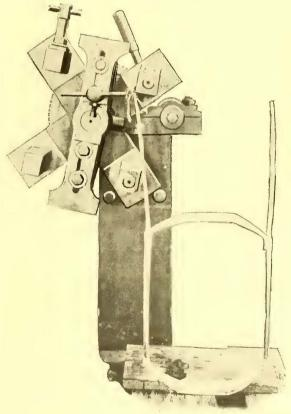
FIG, 6.—ARMATURE COIL WINDER FOR WESTINGHOUSE 49 MOTORS
