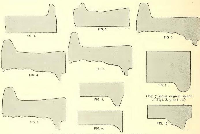
SECTIONS OF STEEL WHEELS WORN ON FLANGE OR TREAD
