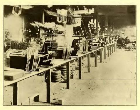
FIG. 10.-PRESSES FOR INSULATING ARMATURE COILS
