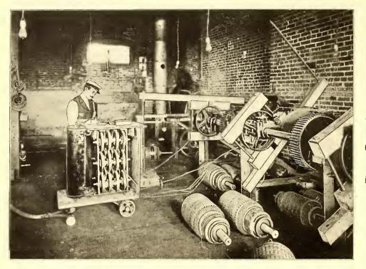
FIG. 12.-TESTING FRAME SCALES AND MOVABLE CONTROLLER WITH LEADS AND PLUGS
