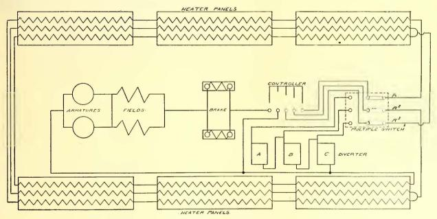
FIG. 4.-DIAGRAM OF WIRING
