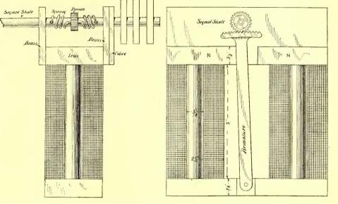
of the magnetic field, and the pull be- FIG. I.-SECTIONS OF ELECTRO MAGNET USED IN OPERATING BLOCK SIGNAL SYSTEM
