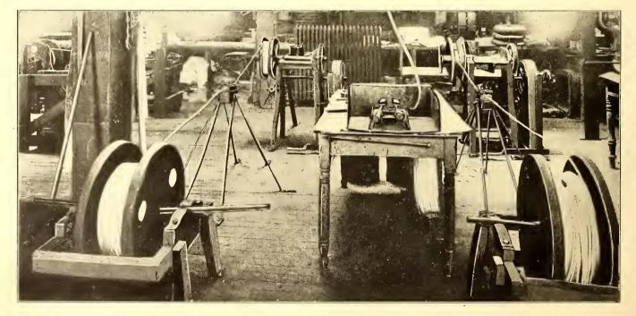
FIG. 9.-FIELD COIL WINDERS
