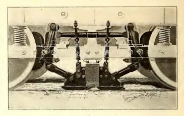
FIG. 2.-VIEW SHOWING METHOD OF ATTACHING BRAKE, TO CAR
