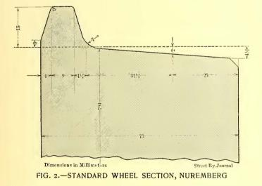
in consequence of the smaller leverage, constantly slides a little, and its thick flange does not permit an equalization. The flange of the small wheel then always travels against the carrying rail, while that of the larger grinds against the guide rail. The wear then assumes the form shown in Fig. I. At the same time the entire truck frame is twisted, as a rule, at an angle to the track, and the wheels diagonally opposite each other show equal forms of wear, although to a smaller extent.
