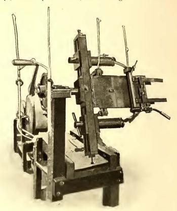
FIG. 2.—ARMATURE COIL WINDER FOR G. E. 57 AND OTHER MOTORS, COIL SPREAD READY TO TAKE OUT
