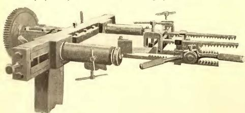
FIG. 3.—ARMATURE COIL WINDER FOR G. E. 57 AND OTHER MOTORS, SHOWING DETAILS OF RACK AND PINION, DIES, ADJUSTMENTS, ETC.
