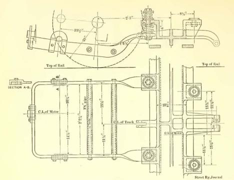
FIG. 24.-MOTOR SUSPENSION OF DOUBLE TRUCK
