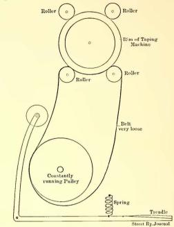
FIG. 8.—DEVICE FOR DRIVING TAPING MACHINE
