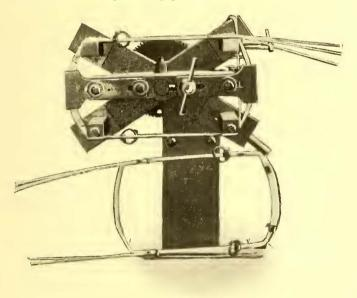
FIG. 4.—ARMATURE COIL WINDER FOR WESTINGHOUSE 56 MOTORS. COIL JUST COMPLETED
