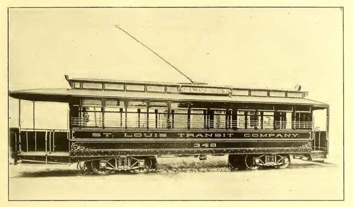
FIG. 20.-NEW SPLICED CAR WITH DETROIT PLATFORM
