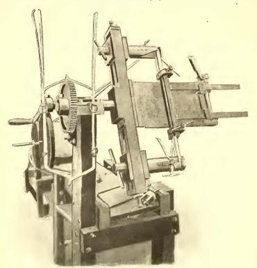
FIG. 1.—ARMATURE COIL WINDER FOR G. E. 57 MOTORS. GENERATOR COIL WOUND AND SET FOR SPREADING
