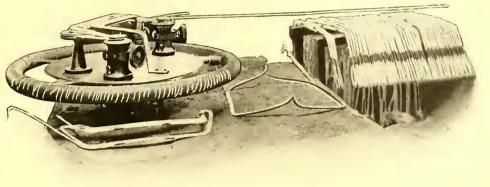
FIG. 5 .- ARMATURE COIL WINDER FOR G. E. 800 MOTOR
