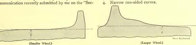
FIG. 1.-WEAR PRODUCED WHEN WHEELS ARE OF DIFFERENT DIAMETER
