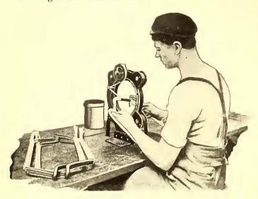
FIG. 7.-COIL TAPING MACHINE
