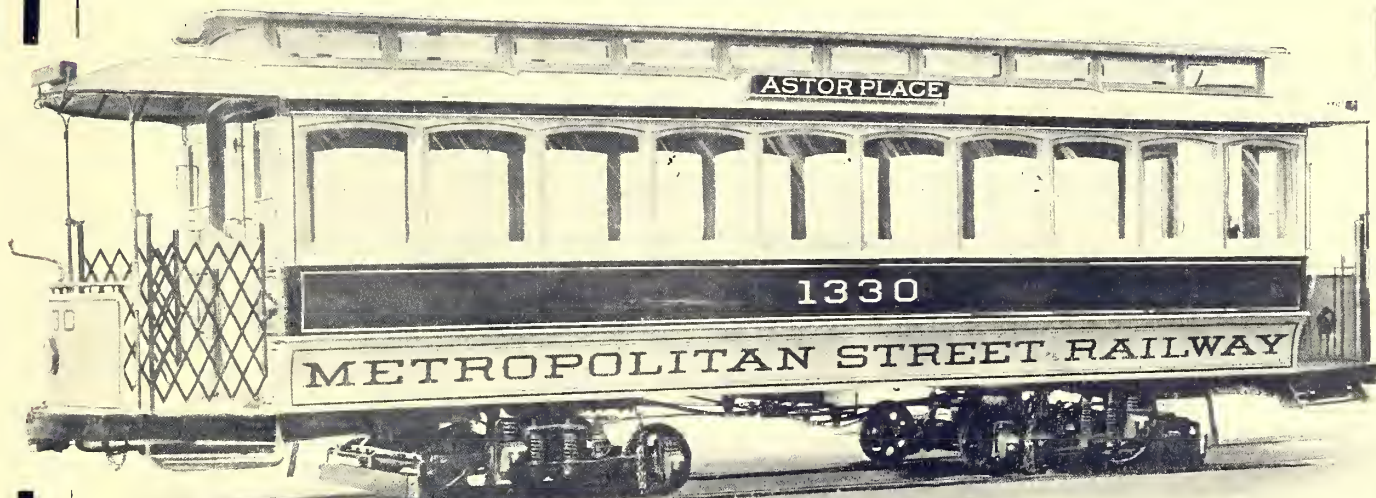
Car of the Metropolitan Street Railway of New York mounted upon Eureka Maximum Traction Trucks.
