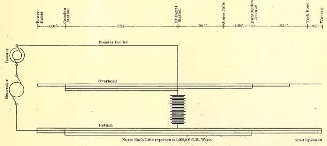
DIAGRAM OF BOOSTER AND LINE FEEDERS
