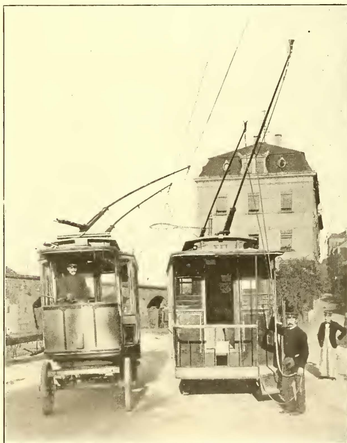
FIG. 4.—TWO CARS PASSING BY REMOVING POLES OF ONE CAR FROM OVERHEAD WIRES
