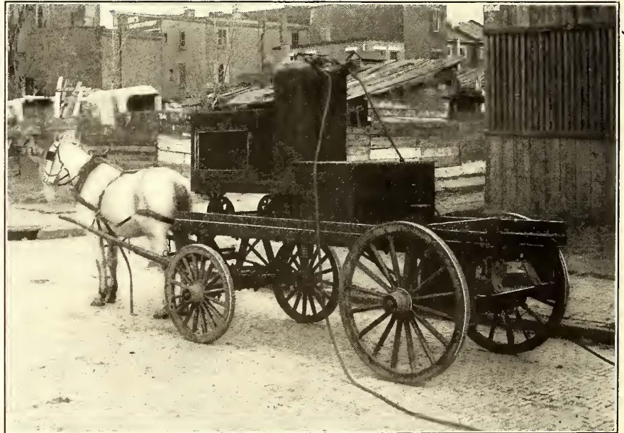
FIG. 10.—COMPRESSING APPARATUS FOR PNEUMATIC RIVETER
