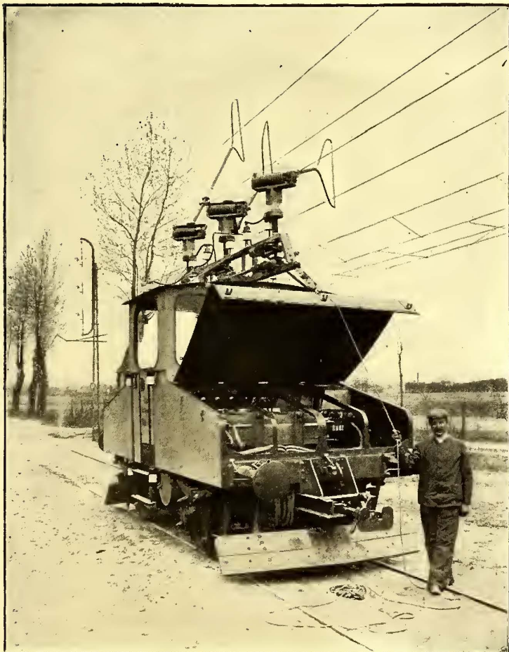
MODIFIED FORM OF CONTACT DEVICE USED IN TESTS AT GROSSLICHTERFELDE
