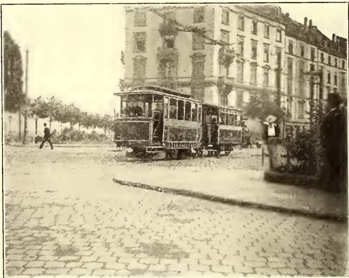
SUPPLY TUBE CONDUCTOR AT FRANKFORT. THE VIEW SHOWS A CROSSING OF THIS OLDEST FORM OF TROLLEY SYSTEM WITH THAT OF THE MODERN BOW TROLLEY
