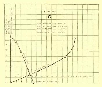
FIG. 1.—TIME AND DISTANCE CURVES FOR EMERGENCY STOPS
