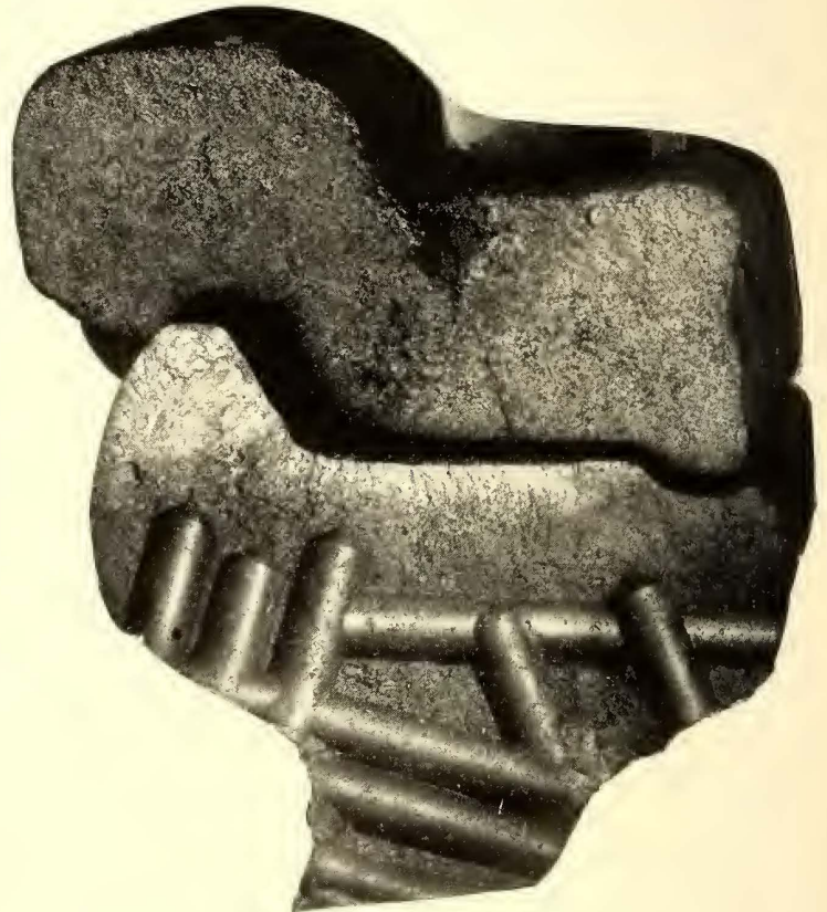
FIG. 1.—WHEEL WITH NARROW CHILL AND CUT BY BRAKE-SHOE
