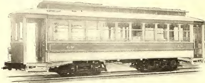
FIG. 1.—DOUBLE VESTIBULE, SEMI-CONVERTIBLE CAR FOR ONEIDA
