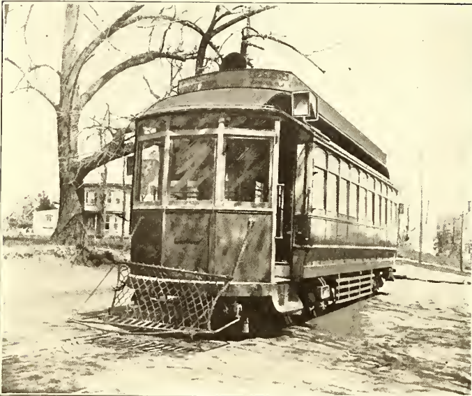
FIG. 1.—CAMDEN CAR EQUIPPED WITH RAILWAY MOTOR VENTILATOR
