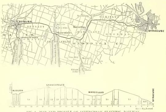
FIG. 1.-MAP AND PROFILE OF INTERURBAN ELECTRIC RAILWAY
