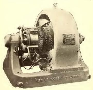
"G" TYPE MACHINE, COMMUTATOR END
