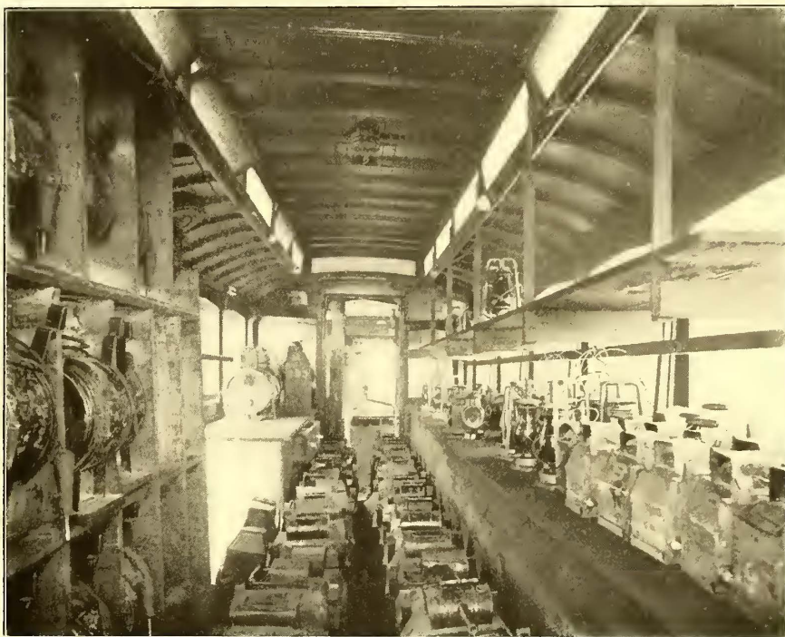
INTERIOR OF LAMP CAR USED FOR SUPPLYING HEADLIGHTS AND TAIL LAMPS TO THE CARS AT TERMINALS.
