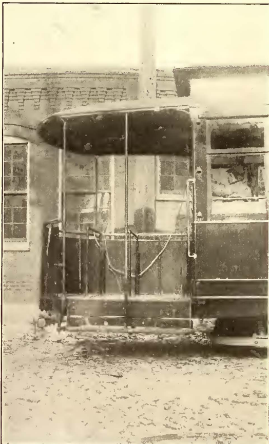
FIG. 2.—LONG PLATFORM WITH TWO RAILINGS IN ST. LOUIS
