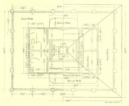
FIG. 2.-PLAN OF COMBINATION WAITING AND SUB-STATION BUILDING
