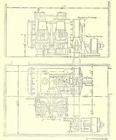
FIG. 18.-PLAN AND END ELEVATION OF CONDENSER PUMPS
