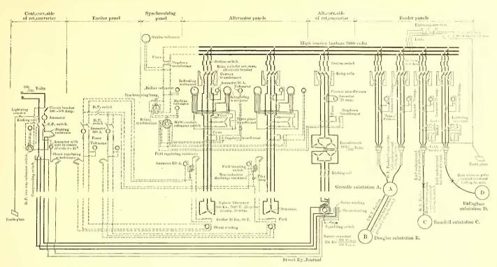
FIG. 10.-DIAGRAM OF SWITCHBOARD CONNECTIONS AT LAXEY GENERATING STATION
