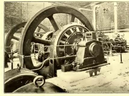
DIRECT-CONNECTED GENERATING SET, 200-KW CAPACITY
