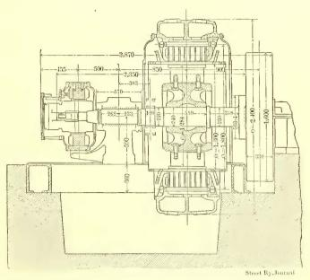
FIG. 5.-ALTERNATOR AND EXCITER
