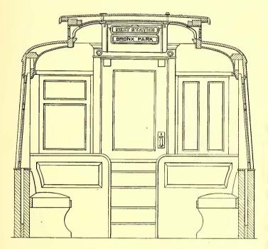
FIG. 1.—CROSS SECTION OF CAR, WITH PNEUMATIC STATION INDICATOR
