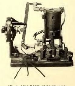
FIG. 3.—AUTOMATIC CUT-OFF WITH COVER REMOVED
