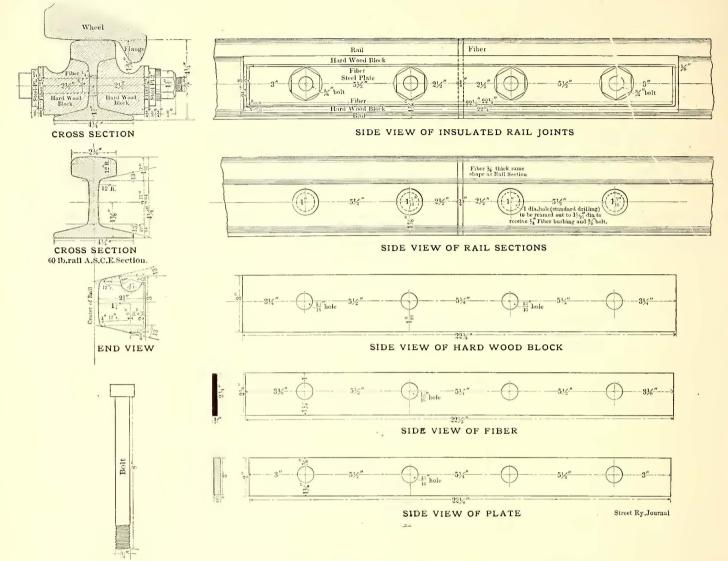
FIG. 3.-INSULATING RAIL JOINTS USED IN CONNECTION
