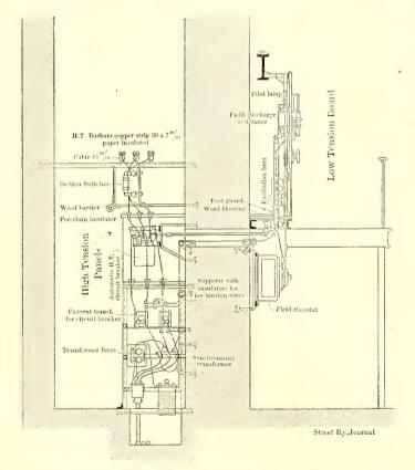
FIG. 14.—SECTION THROUGH ALTERNATOR PANEL AT LAXEY
