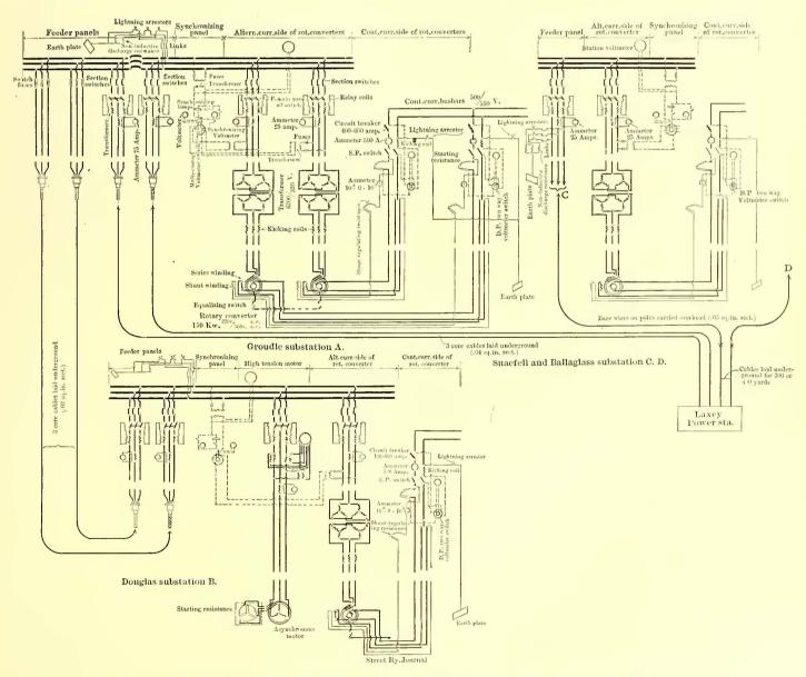
FIG. 13.--DIAGRAM OF SWITCHBOARD CONNECTIONS AT BALLAGLASS SUB-STATION
