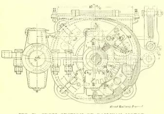
FIG. 21.-CROSS SECTION OF RAILWAY MOTOR
