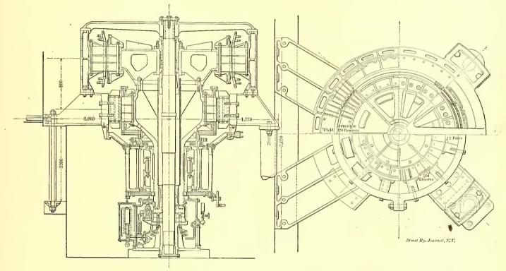
FIG. 1.-DETAILS OF VERTICAL MOTOR GENERATOR SET
