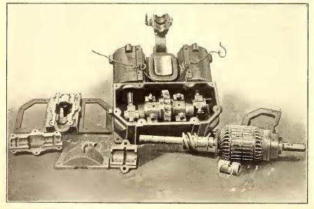
FIG. 2-TOP FIELD AND ARMATURE OF MOTOR REMOVED
