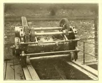
TRAVELER OF OVERHEAD CRANE IN POWER STATION
