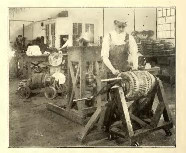
FIG. 9.—ARMATURE SHOP, BAND WIRING APPARATUS AND ARMATURE HORSES AND WAGONS, IN BACKGROUND FIELD-COIL DEPARTMENT
