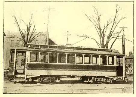
FIG. 10.-STANDARD DOUBLE-TRUCK CAR
