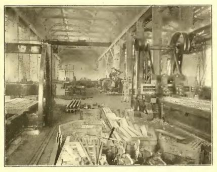
FIG. 10.-MACHINE SHOP, VIEW DOWN CENTRAL BAY, SHOWING TRAVELING CRANE, TWO PLANERS, ETC.
