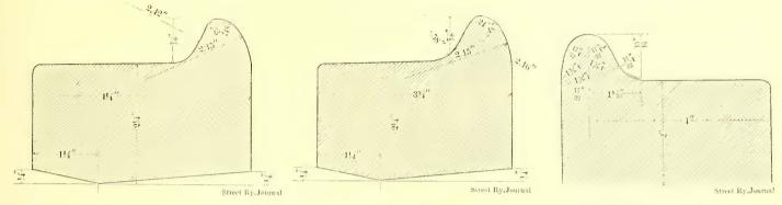
FIGS. 1, 2 AND 3.-SECTIONS OF TIRES OF FUSED WHEELS USED ON ELECTRIC INTERURBAN RAILWAYS
