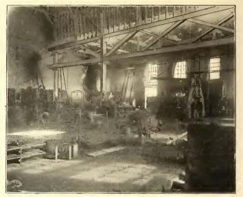
FIG. 14.—BLACKSMITH SHOP, SHOWING AT RIGHT 3000-LB. STEAM HAMMER, AND BACK OF THAT, OIL FURNACE FOR AXLE AND OTHER FORGINGS
