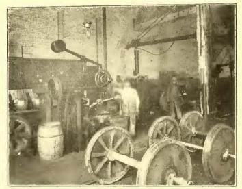
FIG. 12.—MACHINE SHOP, SHOWING WHEEL PRESS AND WHEEL BORING MACHINE, ALSO AT LEFT, TYPE OF WASH BASIN USED IN SHOP
