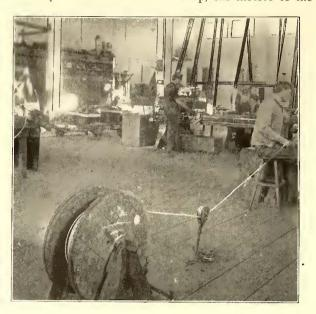
FIG. 7.—ELECTRIC DRYING OVEN IN ARMATURE SHOP, WITH TYPE OF ELECTRIC CAR HEATER SHOWN ON FLOOR
