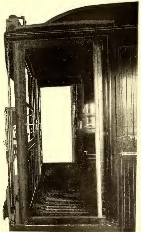
VIEW ACROSS ENCLOSED PLATFORM, SHOWING LARGE SIDE DOOR OPENING
